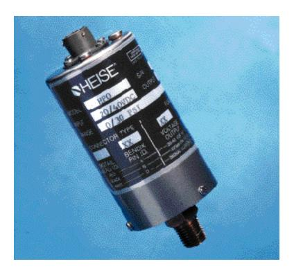
The Heise® HPO precision pressure transducers combine the timeproven precision and stability of the Heise photo-optic sensor with an all-new SMD electronics circuit. These features provide exceptional performance with accuracies of ±0.05% of span or better. The patented photo-optic sensor has no moving parts, linkages, epoxies or O-rings which can contribute to drift and instability.
